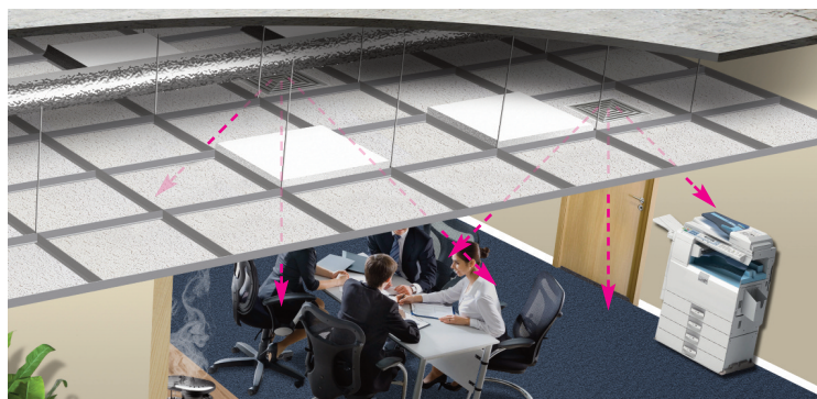
Fig 2. An example of noise generated in ceiling voids - air conditioning for example.
