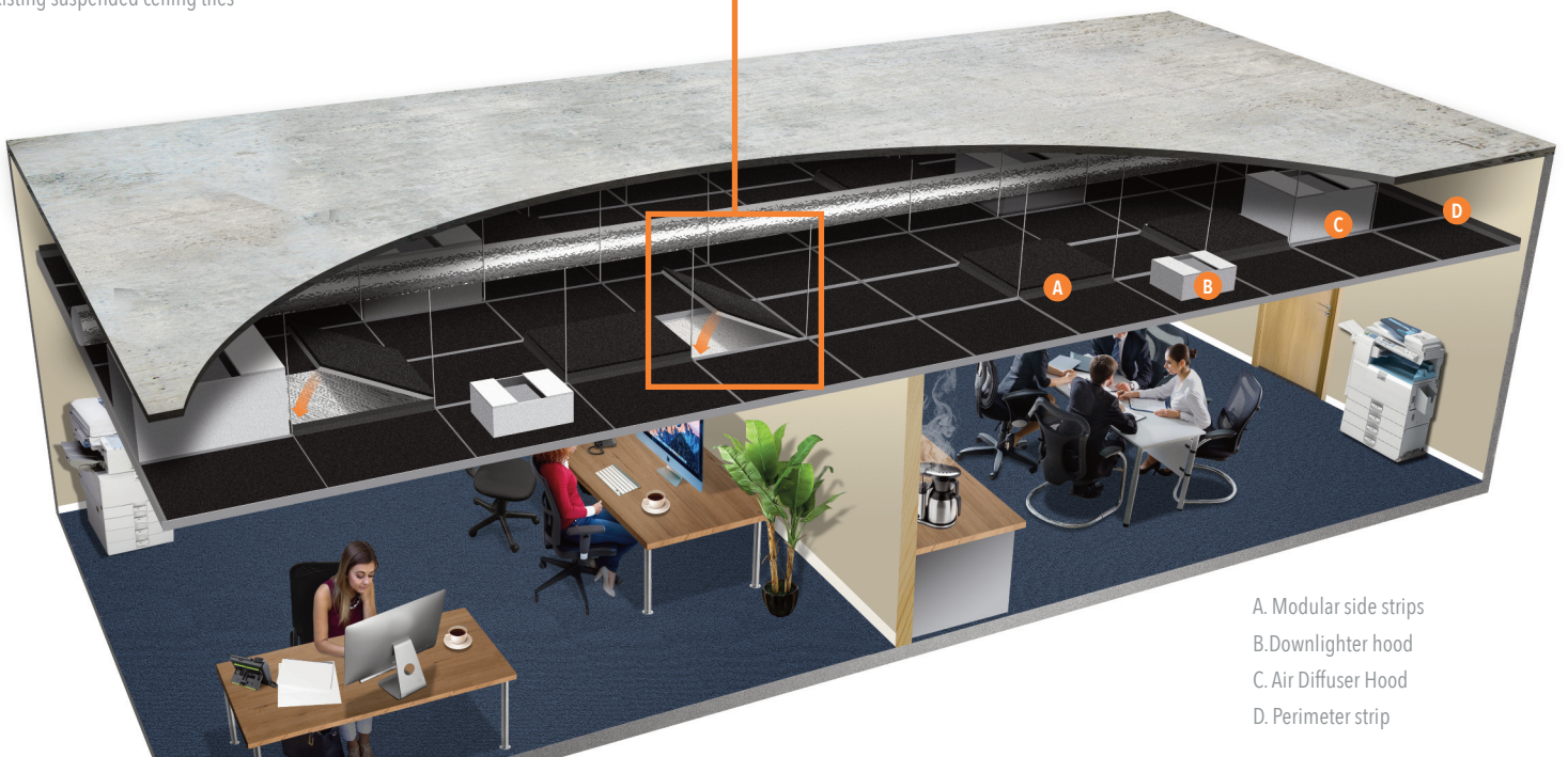
Soundblocker tiles sit on top of existing suspended ceiling tiles
